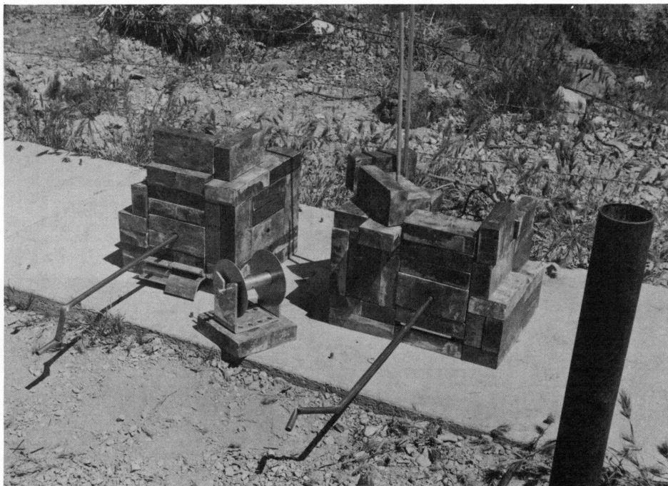
Fig. 2.3—Apparatus for putting wire "spine" on source tubes.
